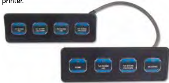
Two 6311-0400-00 connected with OL40-2020-00 cable assembly
