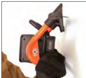
Spike into Drywall
